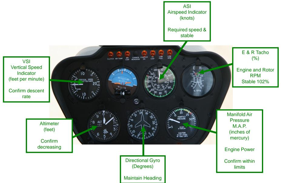
Aim: To learn how to descend at a given speed, T.E.M.: Lookout, Carb Heat, T's & P's, Direction, Control Handover
